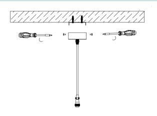
5. After completing step 4, lock the ceiling plate onto the mounting bracket.
