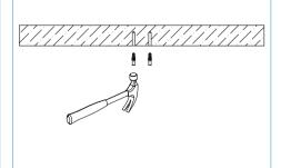
2. Use a hammer to knock the expansion tube into the hole.
