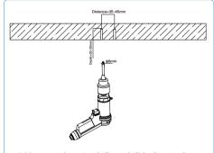
1.Use an electric drill to drill holes in the ceiling. The drill bit diameter is 6mm, the drilling distance is 35–45mm, and the drilling depth is 30–35mm.
