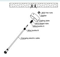
4.1. ①: First remove the nut and gasket on the wire buckle, then pass the M10 threaded tube on the wire buckle through the ceiling plate, and then lock the removed gasket and nut to the threaded tube.
