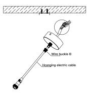
4.2. ①. Pass the hanging electric cable through the wire buckle and connect it to the L, N, GND phase wires at the power grid end (Note: Before electrical connection, the power grid end must be powered off!). ②: Pull the hanging electric cable to the appropriate position. Then lock the wire buckle B.
