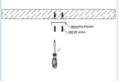
3. Use M4\*25 screws to fix the mounting bracket to the expansion tube on the ceiling.
