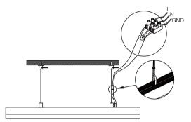
(4) Connect the power supply and complete the installation.
