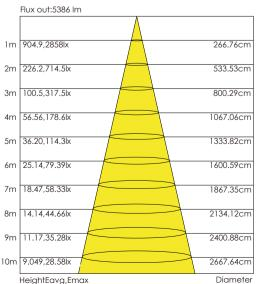
Note: The curve is the illumination area and the average illuminance of the luminaire under different projection distances.
