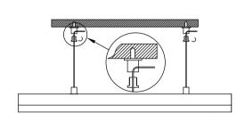
3 Lock the wire sling fixing parts, and fixed the installation length by adjust the wire sling;
