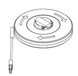
3 When the strip light is stored, the handle needs to be reset to its final state.
