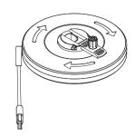
2 Turn the handle 180 degrees, parallel to the turning end cap
