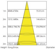
Note: The curve is the illumination area and the average illuminance of the luminaire under different projection distances.
