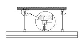
③ Lock the wire sling fixing parts, and fixed the installation length by adjust the wire sling;
