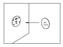
Remove the 3M tape. Fixed in the desired position
