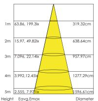
Note: The curve is the illumination area and the average illuminance of the luminaire under different projection distances.
